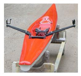
surfing conditions. It makes for easy beaching or dragging up a dock without fear of damage. Since the keel does not go to the stern of the shell, turning the shell in close quarters at slow speed is effortless. The rolled gunwale makes for a strong stiff boat and together with the high bow keeps the water down and the rower dry in rough conditions.
