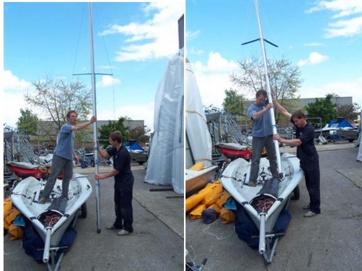
Picture 4.7 Raising the mast.
