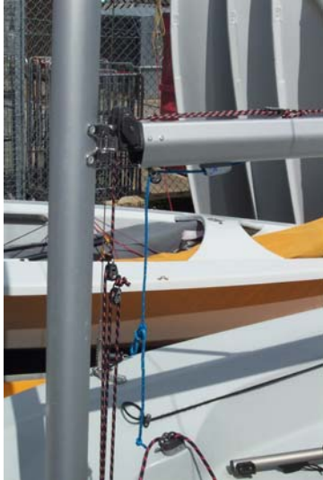
Picture 4.15 The gnav control line.
