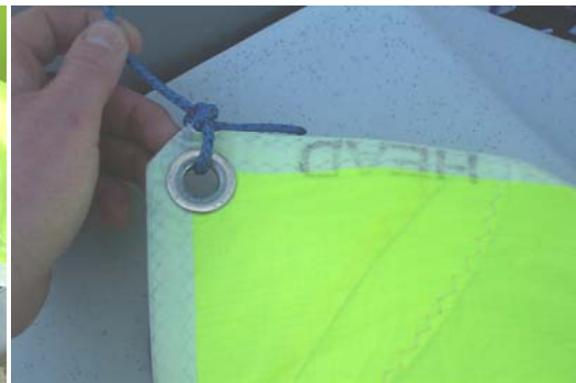
Picture 4.32 The head of the spinnaker.
