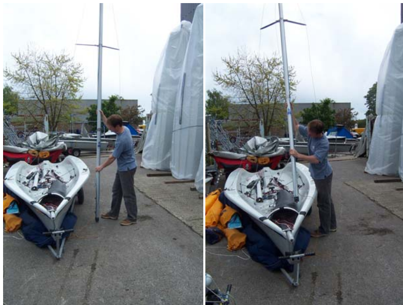
Picture 4.5 Stepping the mast single-handed.
