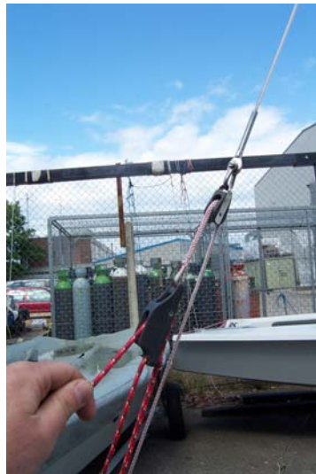
Picture 4.18 Connecting the rig tension.
