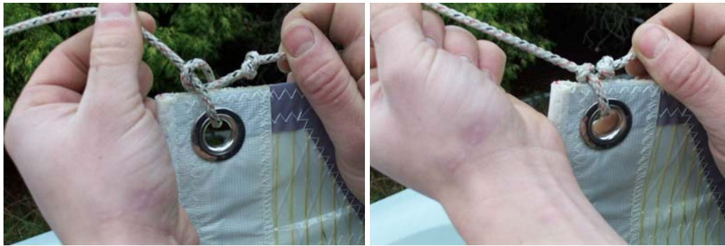
Picture 4.27 Tying the main halyard.
