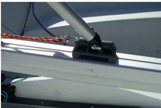
Picture 4.13 Connecting the gnav to the boom.
