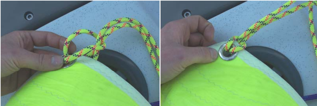
Picture 4.35 Tying the spinnaker sheets.
