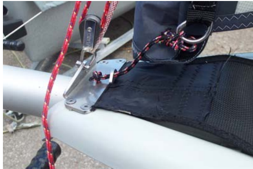
Picture 4.17 The tack of the jib
