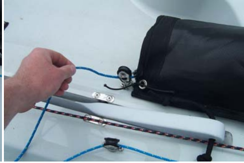
Picture 4.12 The spinnaker downhaul block.
