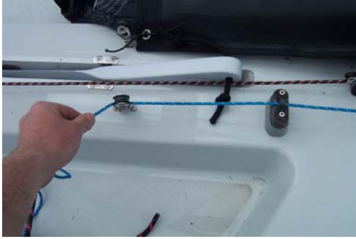
Picture 4.11 The spinnaker halyard cleat.
