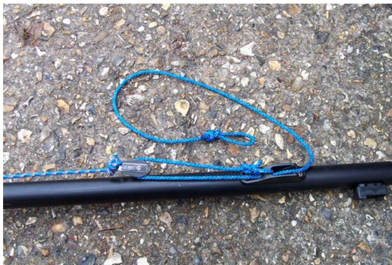
Picture 4.23 The rudder downhaul fitted.
