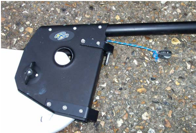
Picture 4.22 The rudder fitted in the stock.
