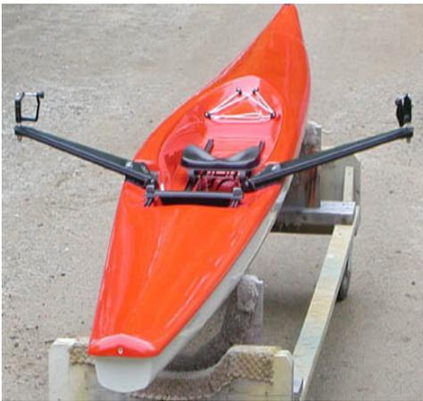
Boat Specs: The Echo weighs about 48 lbs fully rigged and has a suggested weight limit of 260 lbs. Its overall length is 18', has a waterline length 17' 3", a beam at the deck of 26" and a waterline beam of 21".
